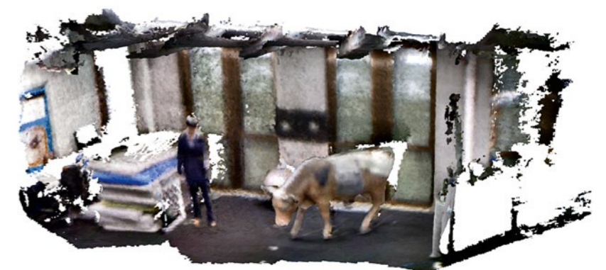
3D reconstruction of the environment by flying robots in realtime, Autonomous Systems Lab, ETH Zurich
