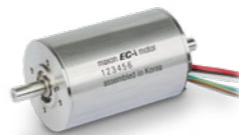
maxon DCX 12 L Ø 12 mm, 2.5 W, precious metal brushes
