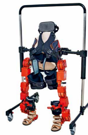
The frame helps to maintain balance, but the exoskeleton can also be used without.
